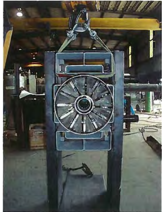
Coen Burner Components Installed In Shop Windbox Mock-up to Ensure Proper Field Fit-up and Demonstrate Installation Procedures to Customer
